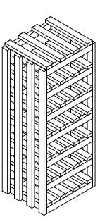
5. Middle Stack and Top Stack rack can be place directly on top.
